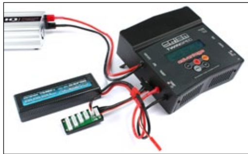
2S LiPo battery with Deans and HX connectors
