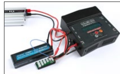
2S LiPo battery with 4mm and 2mm gold tubes connectors
