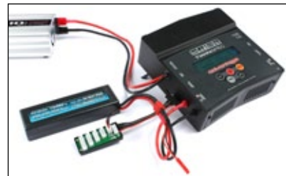
2S LiPo battery with Deans and XH connectors
