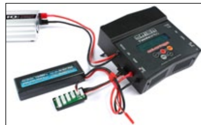
2S LiPo battery with Deans and XH connectors
