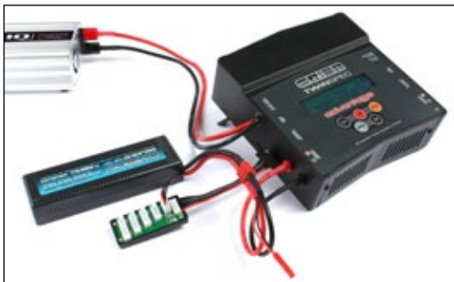
2S LiPo battery with Deans and HX connectors
